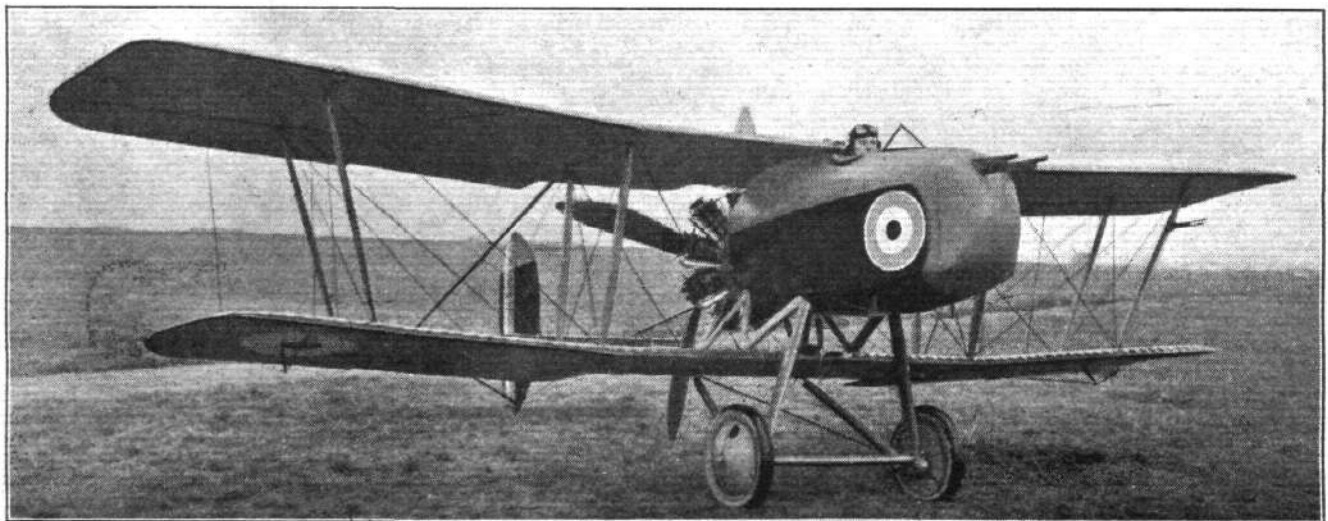
THE VICKERS "VAMPIRE."—This machine, which is a modification of the F.B. 26, is armoured and intended for trench fighting. The engine is a 200 h.p. B.R. 2
